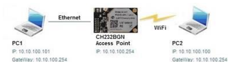
Figure 14: CH232BGN As Access Point
