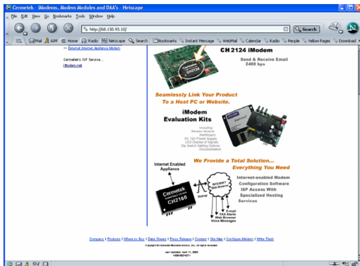
Figure 1B. Lower portion of Cermetek Web page stored in CH2165. This is the window used to access the CH2165 CGI feature. Note the CONFIGURE IMODEM and WRITE FLASH items in the lower right corner.
