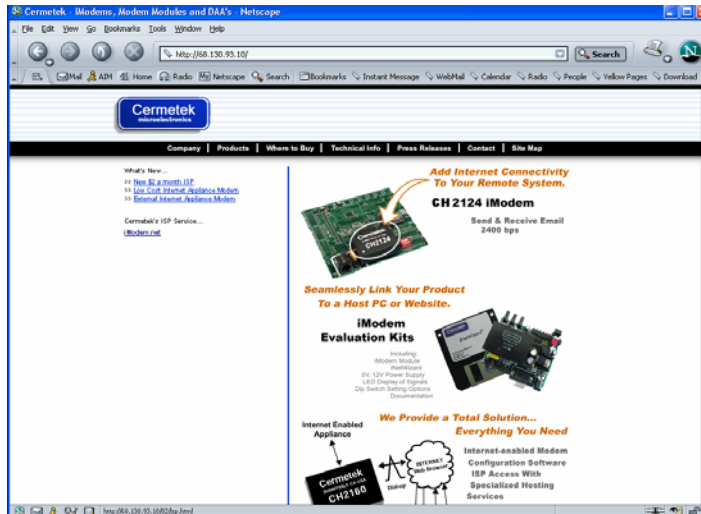
Figure 1A. Upper portion of Cermetek Web page stored in CH2165. This is the window used to access the CH2165 CGI feature.
