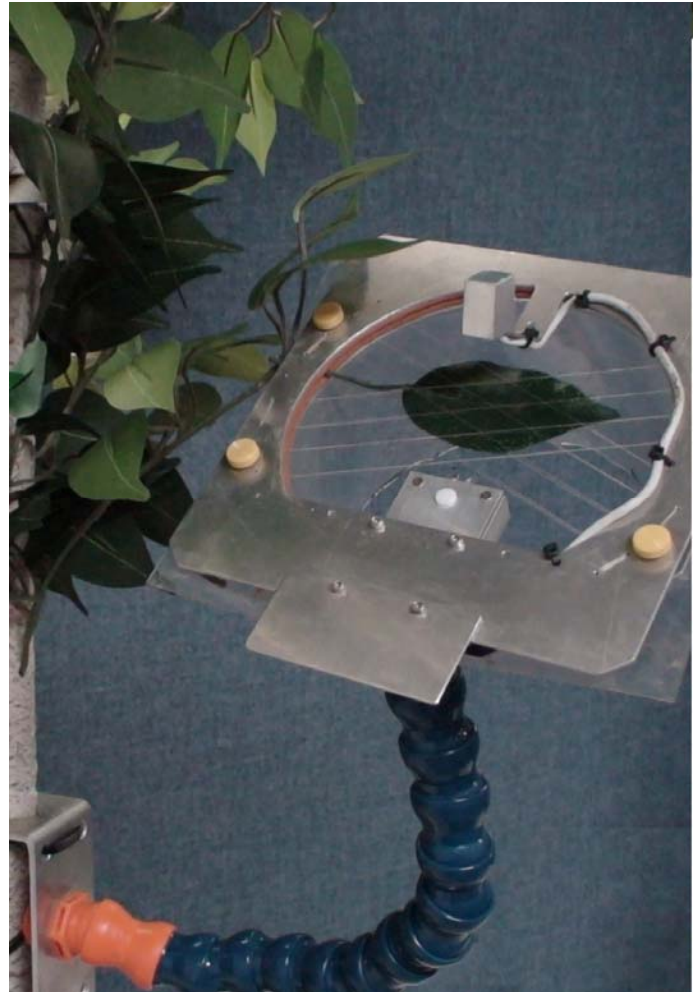
Leaf Placed in Modified Crop Water Stress Index Sensor
