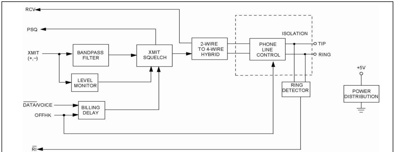
Figure 1: CH1840 DAA Functional Block Diagram
