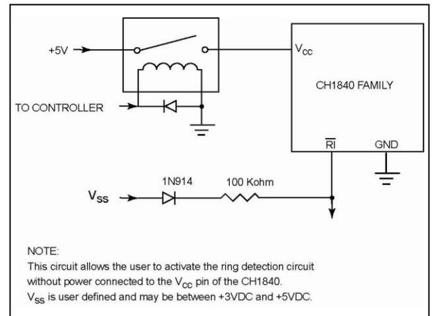
**Figure 2: Low Power Ring Detection**
