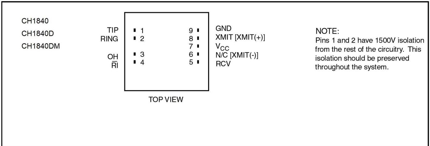
Figure 6: Pin Connections.
