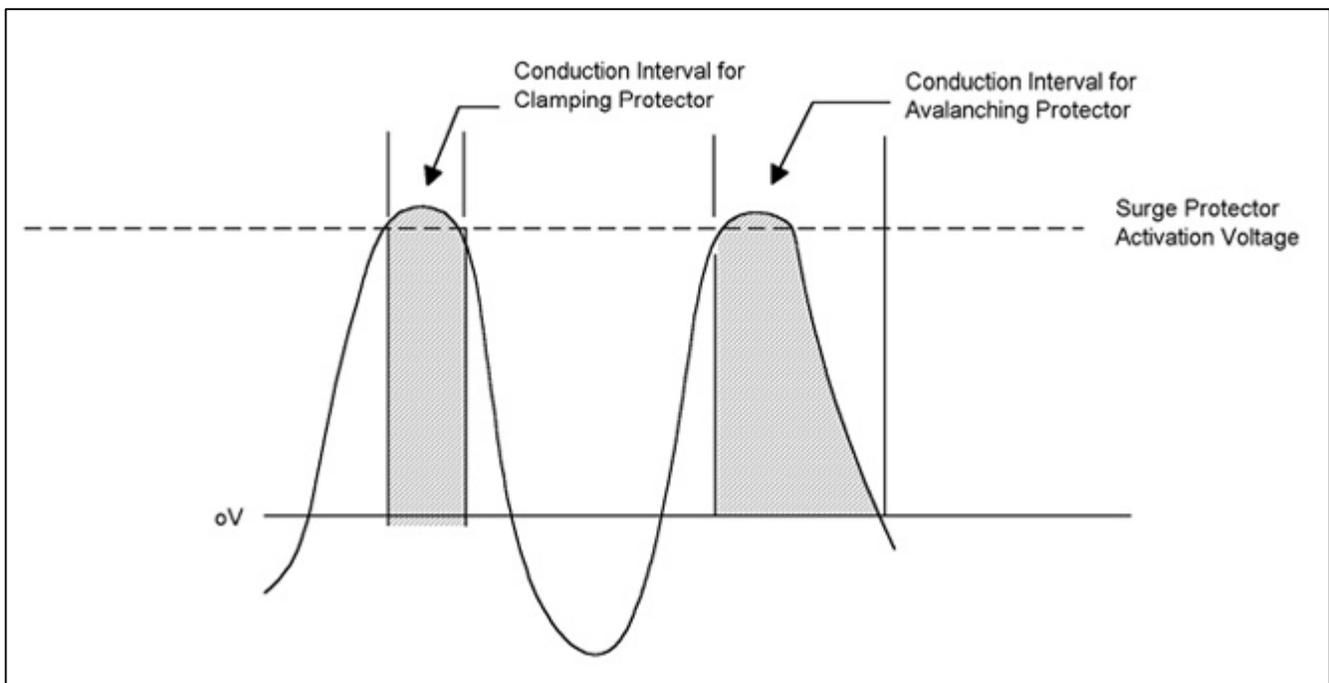
**Figure 8. An expanded view of the ringing signal showing the effect on the ringing conduction interval of a Clamping device vs. an Avalanching device.**
