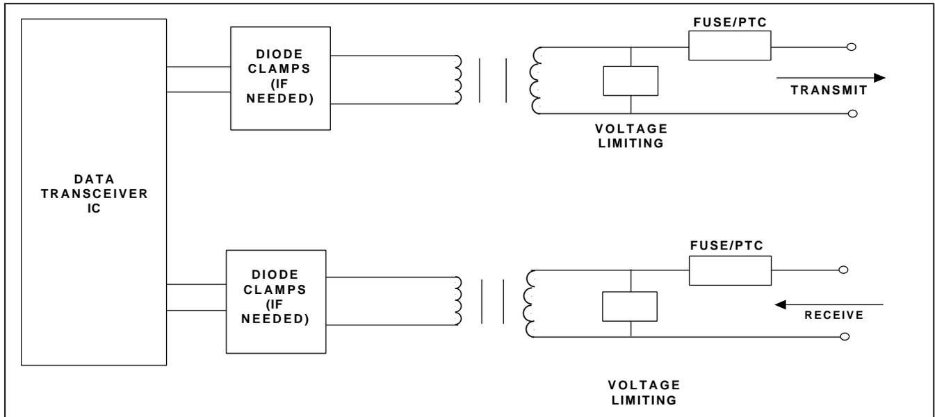
Figure 1. Typical floating T1/E1 interface design. In this figure, the USER side is to the left of the transformer and the TELCO side is to the right of the transformer. Differential surge protection is provided on the TELCO side by voltage limiting devices. The USER side protection functions as additional protection and is useful as protection against residual effects of the stresses. Longitudinal stress is withstood by the transformer dielectric.
