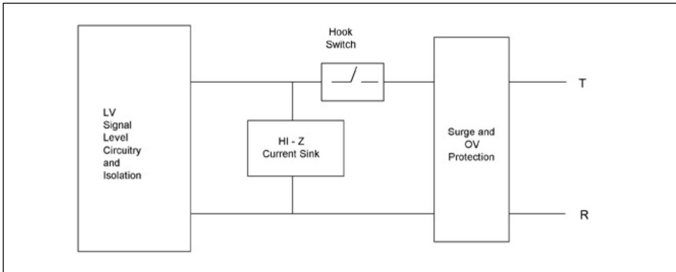
**Figure 3.** A simplified block diagram of an Analog Loop Start terminal device. Note the role of the hook switch. When open, (i.e., on-hook) the hook switch has to withstand the surge voltage up to the level of protection provided by the surge protector as well as any momentary pulses that may “sneak” past the surge protector. When closed (i.e., off-hook), the hook switch must absorb any current pulse caused by a voltage surge.
