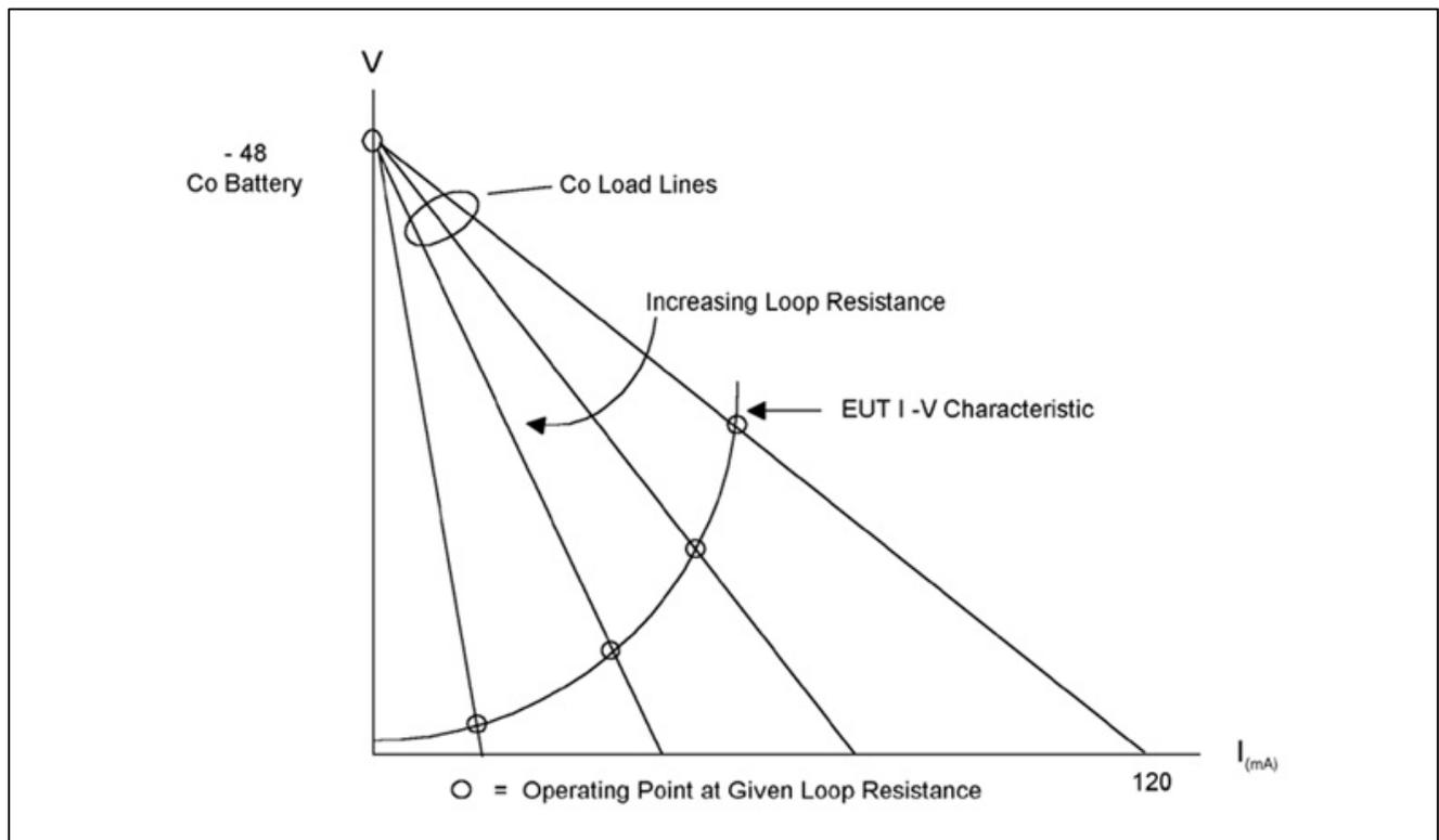
Figure 7: In the off-hook state, the operating point of the terminal equipment is the intersection of the load line of the telephone network and the I-V characteristic of the equipment.
