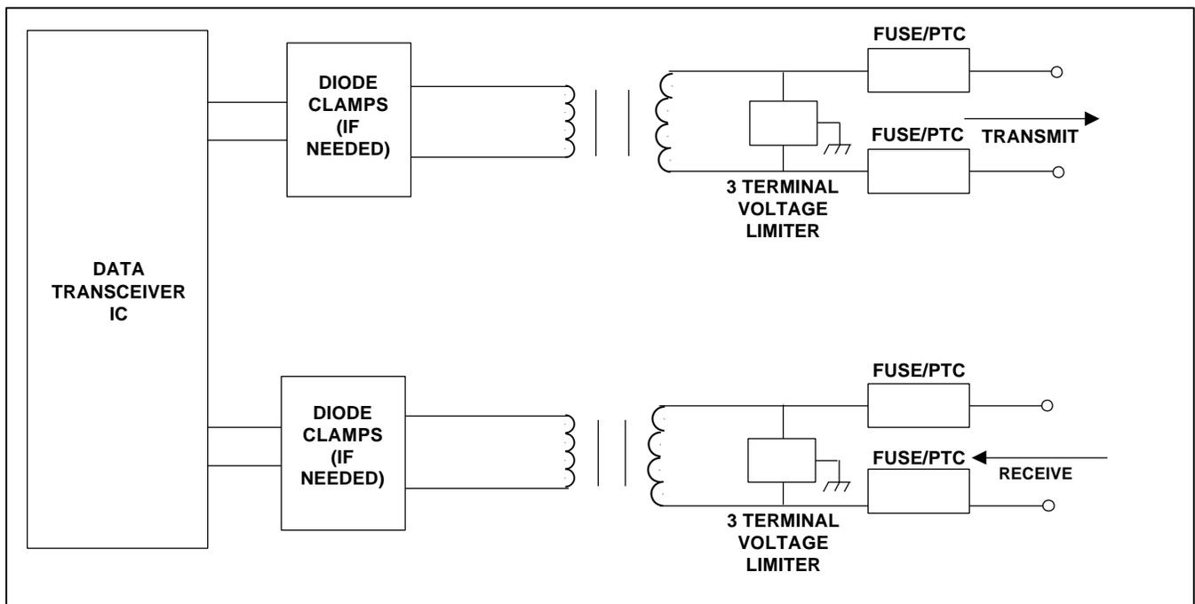
Figure 2. Typical grounded T1/E1 interface design. Differential surge protection functions as in Figure 1, but longitudinal stresses now result in current flow to ground via the third terminal of voltage limiting device. Although grounded voltage limiting is more robust, it requires extra components for proper implementation. Note that the transformer isolation must still meet the longitudinal stresses with the grounded protective component removed.
