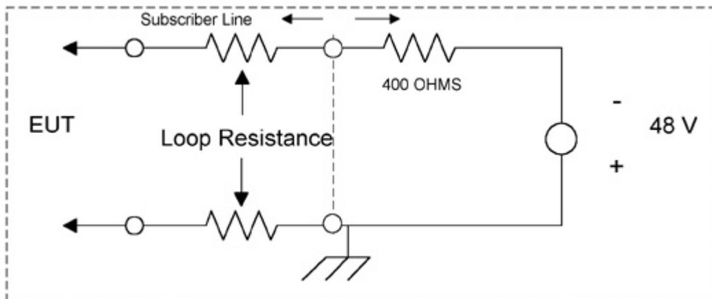
**Figure 5. A simplified DC representation of the PSTN battery and wiring resistance. This representation is adequate for On-Hook analysis.**
