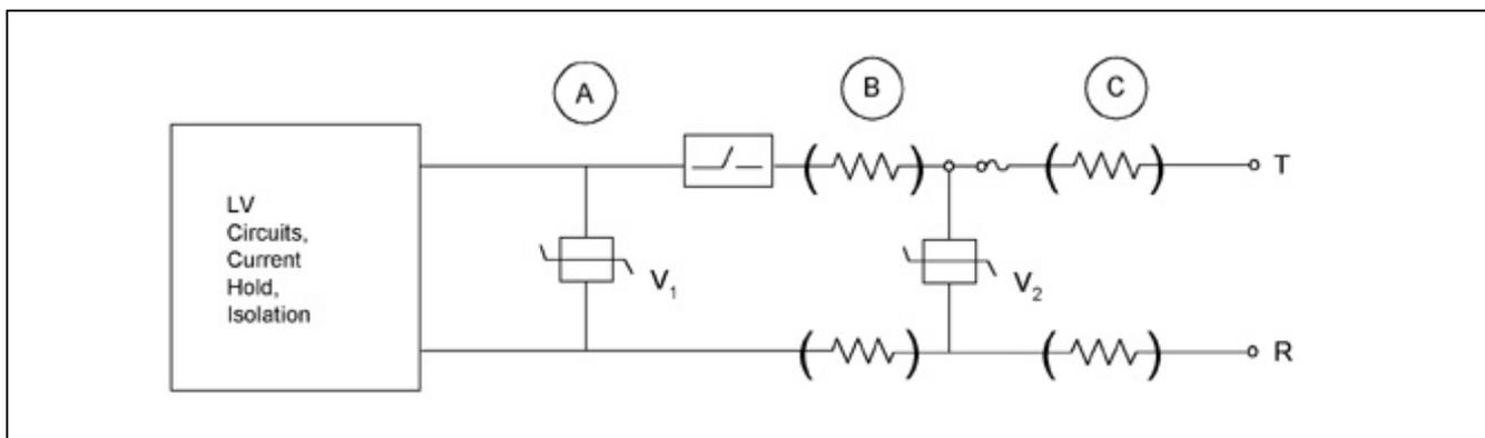
**Figure 4.** A more detailed block diagram of an Analog Loop Start terminal device. Protection of both the hook switch and the low voltage circuitry in the terminal device requires an additional low voltage clamping element ( $V_1$ , circled item A) and may sometimes require additional series resistance (circled items B and C). Note that the greater the resistance added, the smaller the ratio of energy delivered to the terminal device. Device  $V_2$  is the primary voltage protection device.
